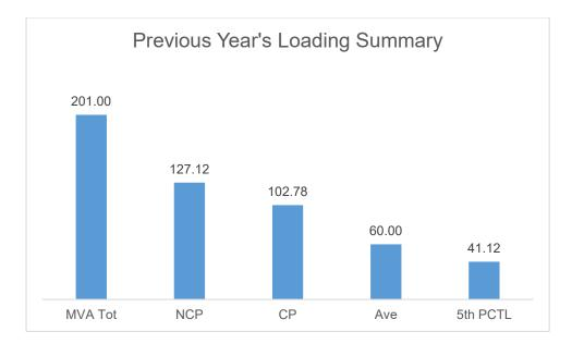
The Non-coincident Peak Demand is 127.12 MW, which is around 63.24% of the total substation capacity of 201 MVA. The load factor or the ratio between the Average Load of 60 MW and the Non-coincident Peak Demand is 47.20% of. A safe estimate of the true minimum load is the fifth percentile load of 41.12 MW which is 32.35% of the Non-coincident Peak Demand.
