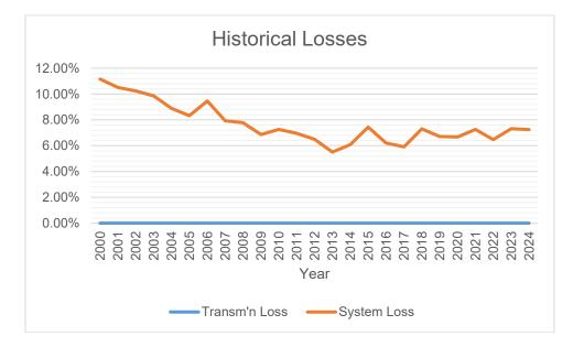
Transmission Loss is always at 0%. MWh Input does not deviate from the MWh Offtake because these are both measured/metered at the Grid Offtake Point (GOTP) located at NGCP Drawdown Substations where DECORP Distribution Substations are being sourced. However, for San Jacinto Substation (MF3MSMNDECO02) which is connected to NGCP San Manuel Substation, transmission loss is also 0% because the Site-Specific Loss Adjustment (SSLA) accounts for the sub-transmission loss and not for the former.
